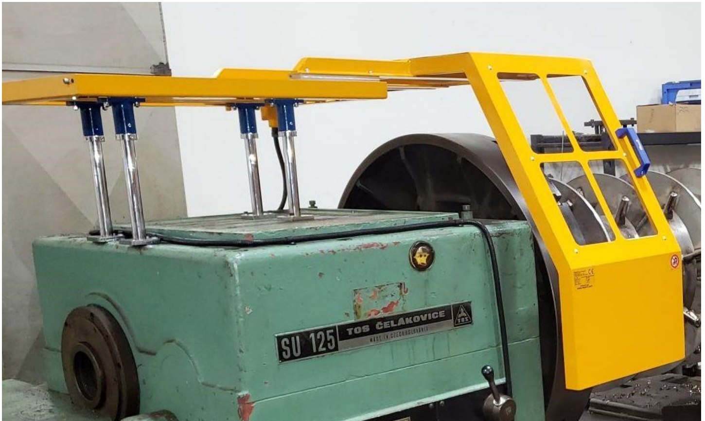
Figure 2: Closup of the blue leg brackets and silver legs.
