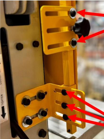
To adjust the shield's distance from the belt, loosen these screws and move the shield to your desired position. Once the shield is properly positioned, tighten the screws securely.
