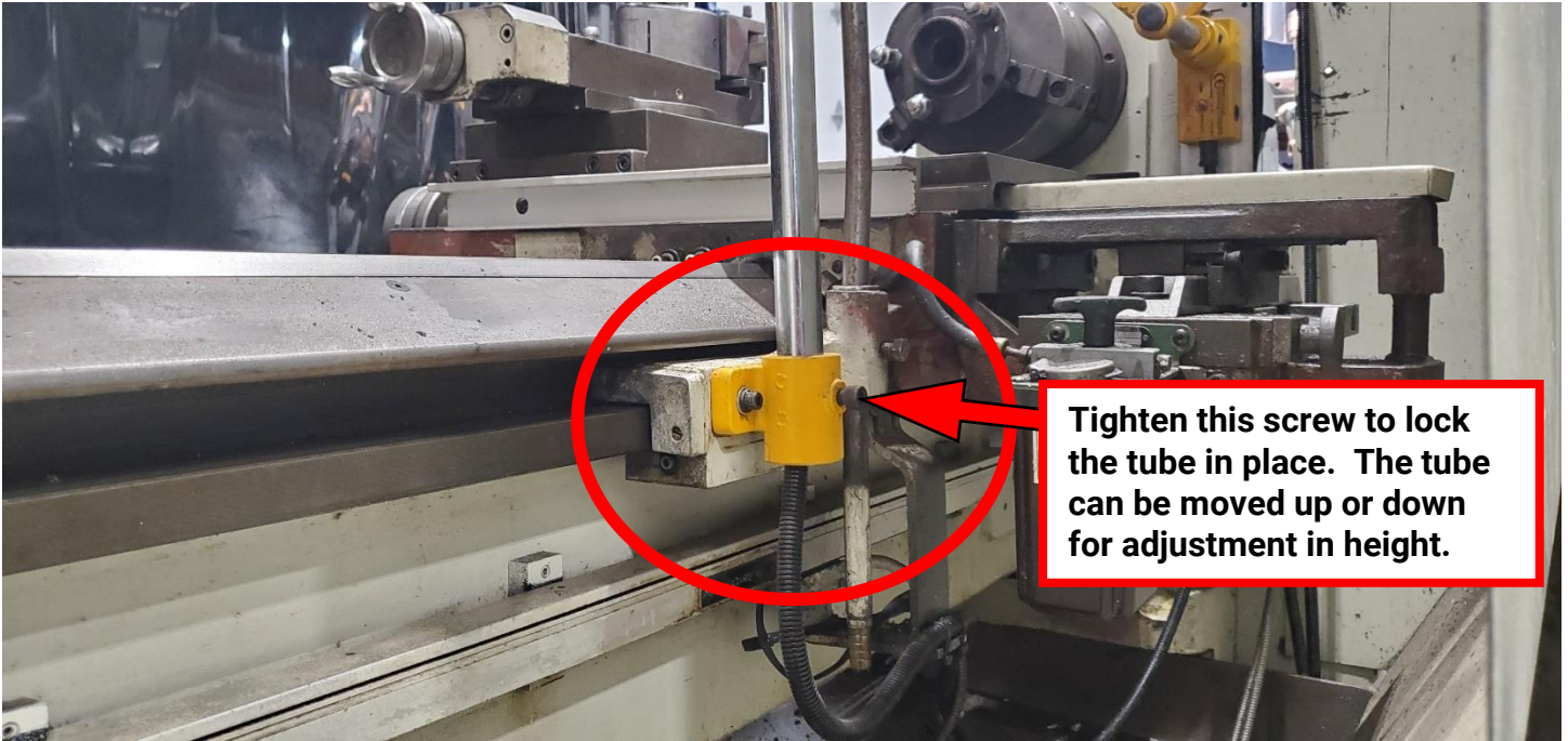
Figure 3: View of the mounting bracket from the back of a lathe.
