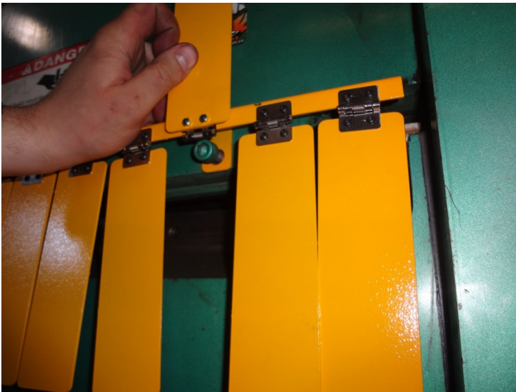
Fig. 10 – Close up of installation bolt. The safety flaps can be lifted up to access the bolts underneath.
