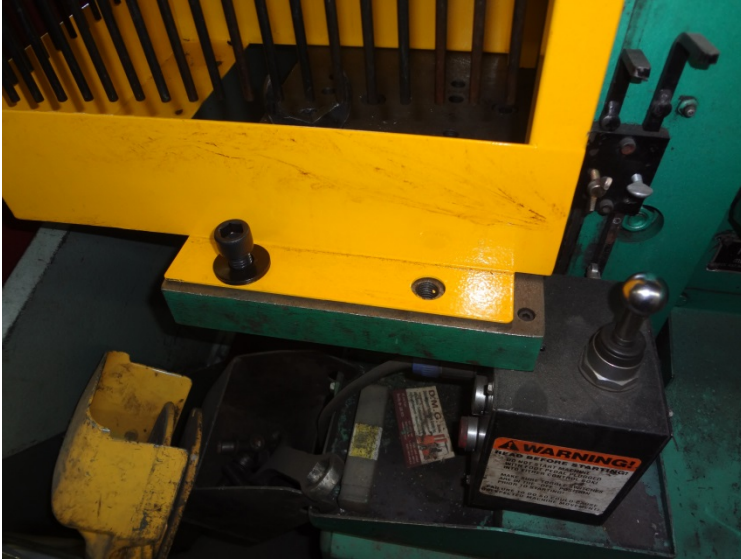
Fig. 11 – Use the four 5/8-11 bolts and washers (provided) to mount the guard directly to the punch side table.
